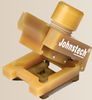
MEMS Manual Actuator lid open showing Johnstech Pad ROL™ 200 Contactor.
