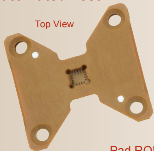
Pad ROL™ 200 Contactor with Alignment Plate for automated handler test.
