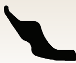
Low-Force XL-2 Contact Profile NiPdAu Configuration
