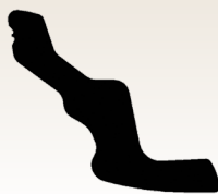
Low-Force XL-2 Contact Profile NiPdAu Configuration
