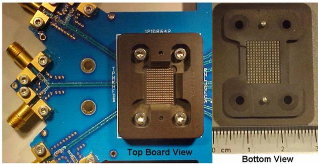
**Figure 17:** Optimized Load Board and Contactor
