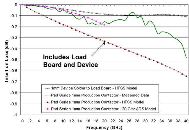
**Figure 19:** Comparing Modeled, Simulated and Measured Results
