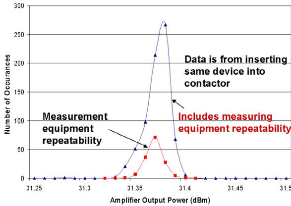
**Figure 4:** Amplifier Output Power Distribution and Repeatability
