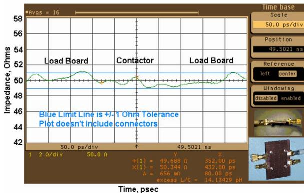
**Figure 7:** TDR Measurement of 1mm Contactor System
