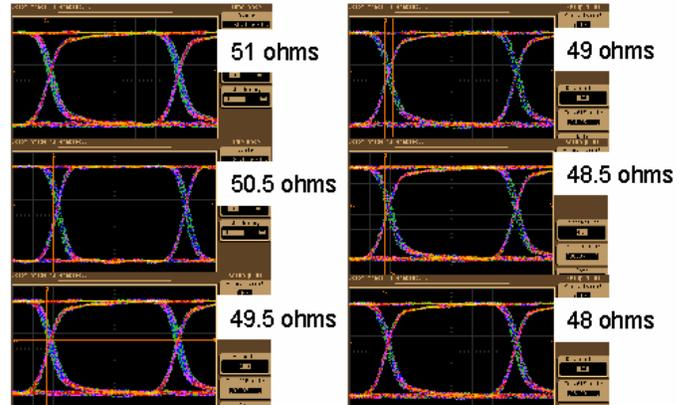
Figure 14; Effects of Trace Impedance on Signal Integrity
