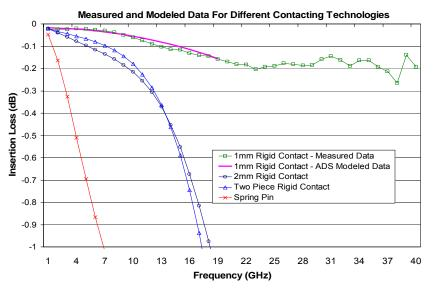
Figure 3. Insertion loss data vs. frequency for various contactors.
