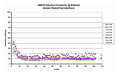
Figure 2. Electrical considerations – contact resistance vs. insertion cycles For 1mm production contactor at ambient temperature
