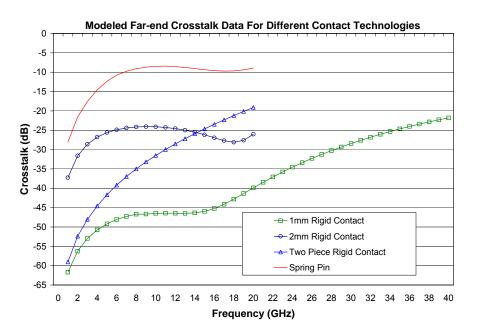
Figure 5. Crosstalk data vs. frequency for various contactors.
