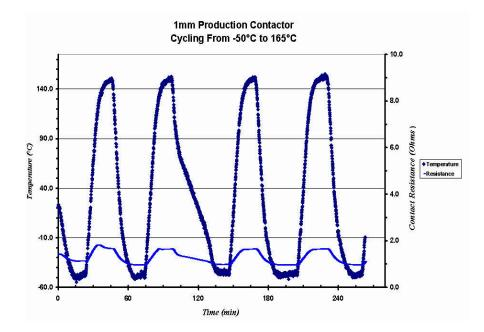
Figure 6. Thermal cycling vs. time for specific 1mm production contactor.
