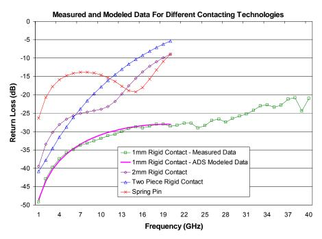
Figure 4. Return loss data vs. frequency for various contactors.
