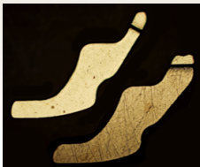
New XM ™ contact (top) Standard contact (bottom)
