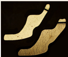
New XM ™ contact (top) Standard contact (bottom)
